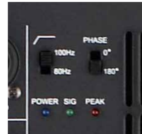
18" sub with built in 80/100Hz crossover and phase switch
