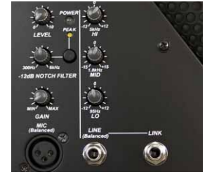
3 band EQ notch filter & mic & line inputs on the front panel - easy access
